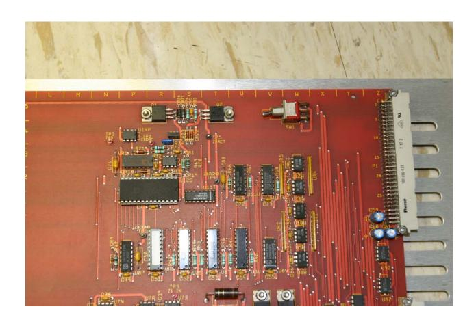
The sw1 is the polarity switch. After flip it, and reinstall the board. Power on the console.
