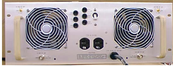
Figure 14. System Power Supply
